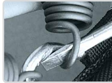
**Replace spring:** Hook the new spring into the frame cleat first. Then use a slotted screwdriver to lever the other end of the spring into the mat cleat.
