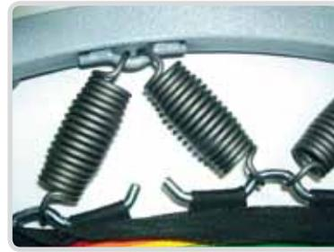
Check that the springs are correctly hooked in the bends of the metal cleats.
